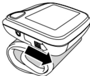
2. Insert 2 AAA batteries with the polarities in the correct direction.
